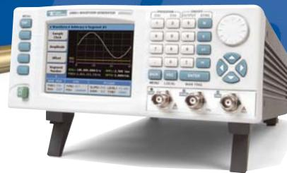
The entire space of the waveform memory is backed up by rechargeable batteries allowing waveforms to be downloaded in the lab and the generator moved to another location for field operation.
